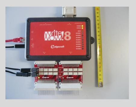
WriteNow! Programmer with demultiplexer module (32 channels with relay
